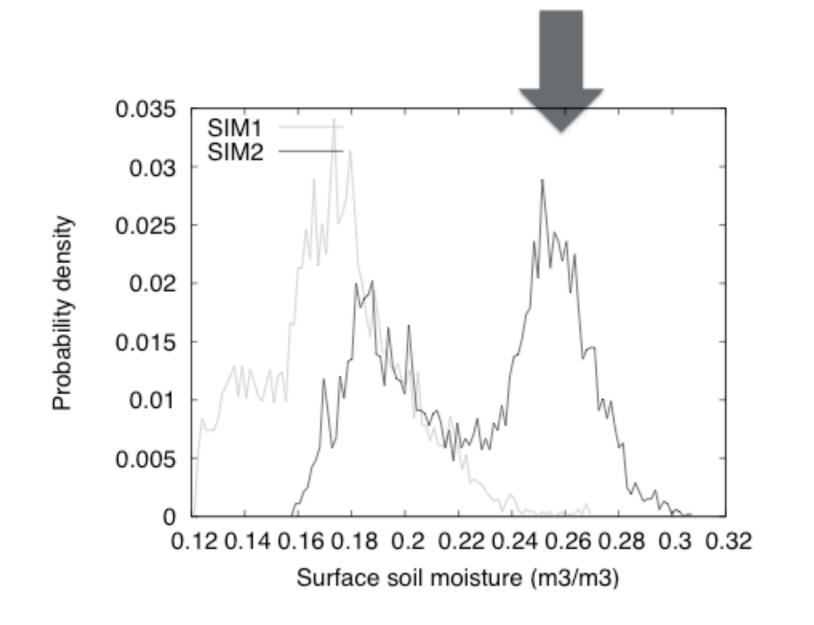
Significant changes in soil moisture distribution due to irrigation with changes in mean, location and symmetry
