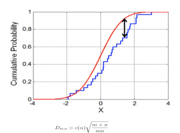
A two-sample Kolmogorov – Smirnov (K-S) test is used to quantitatively compare the PDFs
