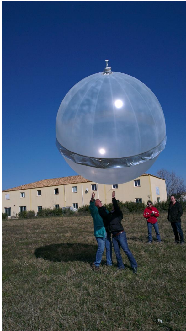
Figure 5: French (a) and German (b) aircrafts deployed during SOP1, R/V Le Provence operated during SOP2 (c) and pressurized boundary layer balloons launched from Candillargues during SOP2 (d) (c). French ATR42 (foreground) and Falcon 20 (background) were based at Montpellier airport and German Do128 was based in Corsica at Solenzara airport. (Source: panels a and d: P. Drobinski; panel b: C. Kottmeier; panel c: I. Taupier-Letage).
