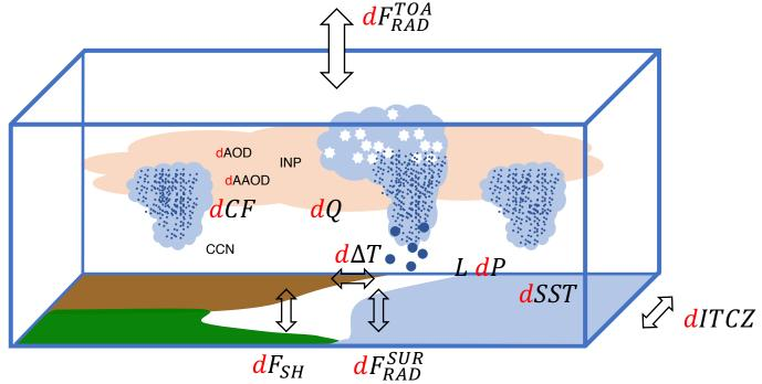
**Direct and indirect aerosol effects via:** surface energy budget, atmospheric diabatic heating, semi-direct effects, regional scale precipitation and monsoon dynamics, sea surface temperature patterns, and hemispheric asymmetry in aerosol radiative effects.
