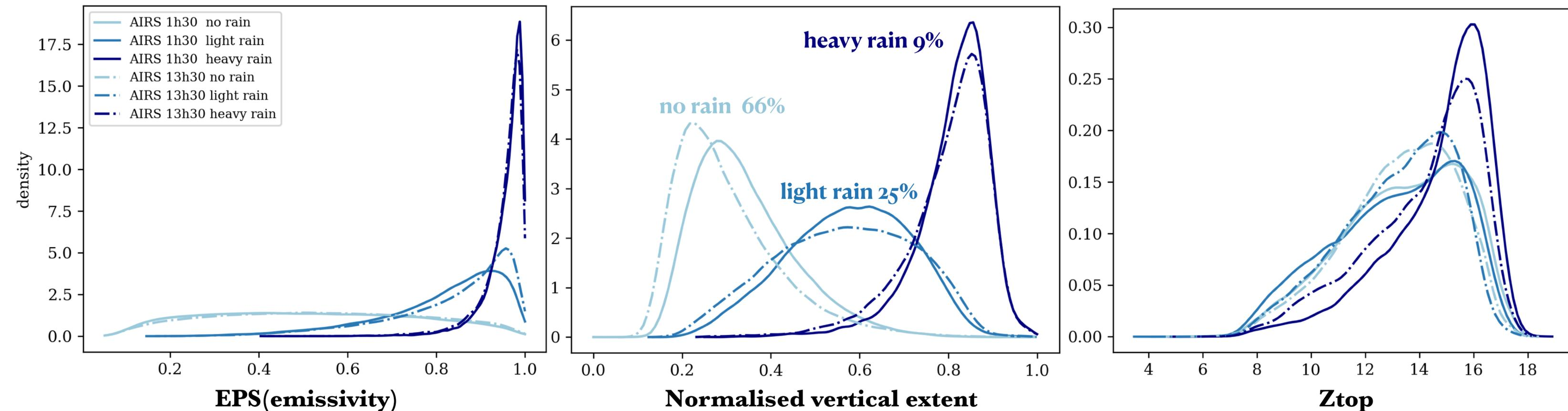
**Rain rate classification from AIRS ML-CloudSat for scene identification:** no rain, light rain, heavy rain
