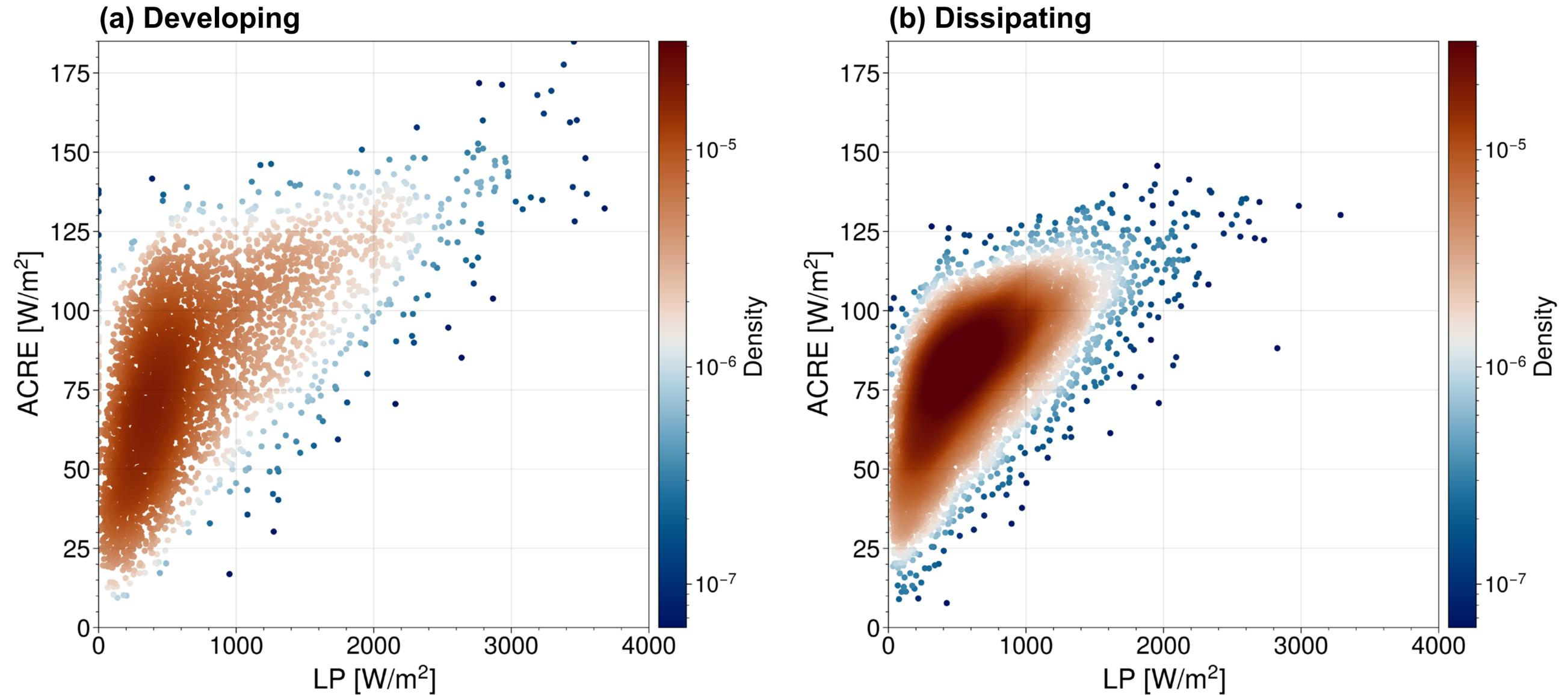
A broad scattering is in the LP-ACRE space of MCSs in the developing stage and a narrower distribution of MCSs is in the dissipating stage.
