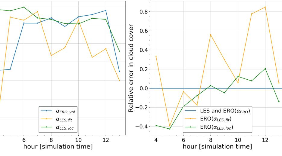
• Left : using the overlap parameter computed on the LES on consecutive cloud layers or by fitting an exponential to the data can lead to a significant error in cloud cover. • Right : comparison for the cloud and total albedo and cloud cover for different reconstructions: vertical subgriding can be used to compensate an initial coarse vertical resolution, if the proper overlap parameter is computed.
