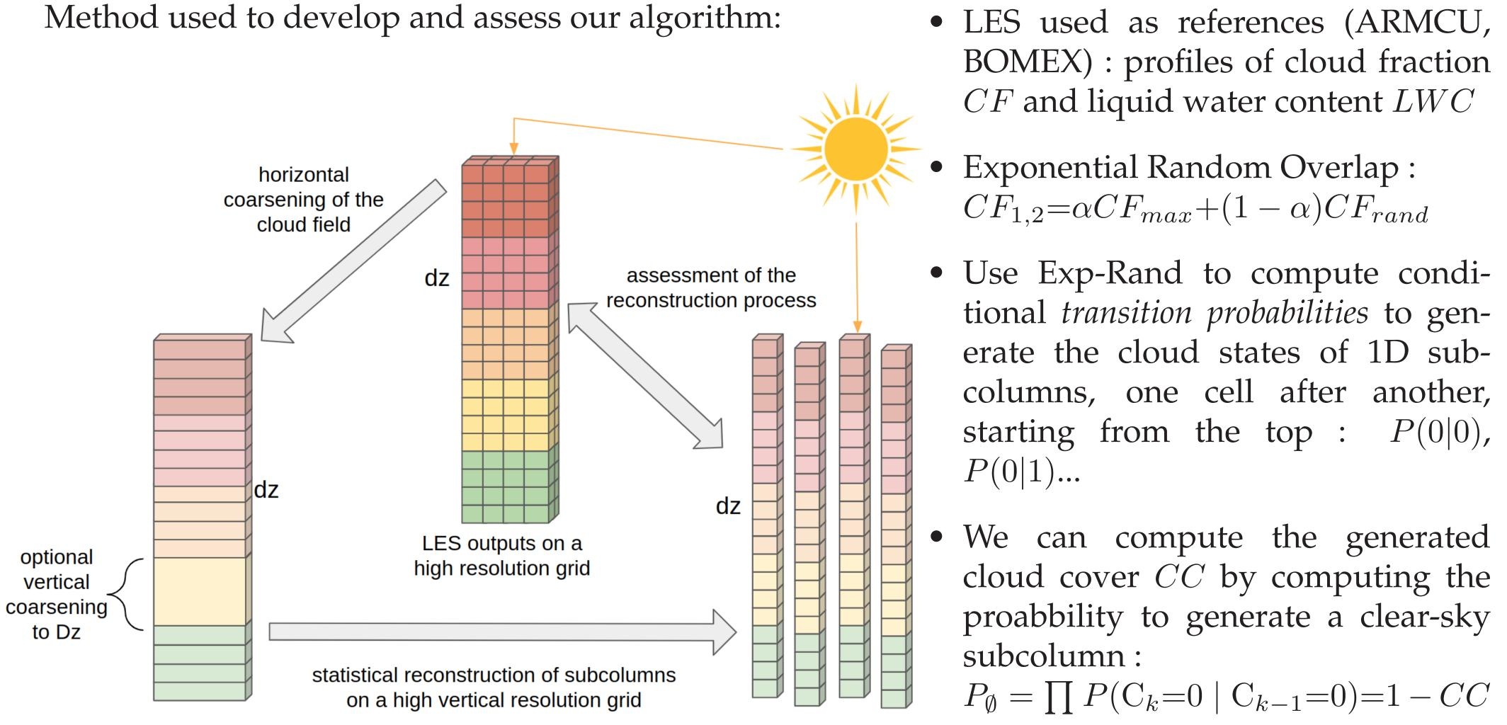
The cloud field of resolution dx = dy = dz = 25m is horizontally averaged into a single column and eventually averaged vertically to a coarse resolution Dz > dz.
